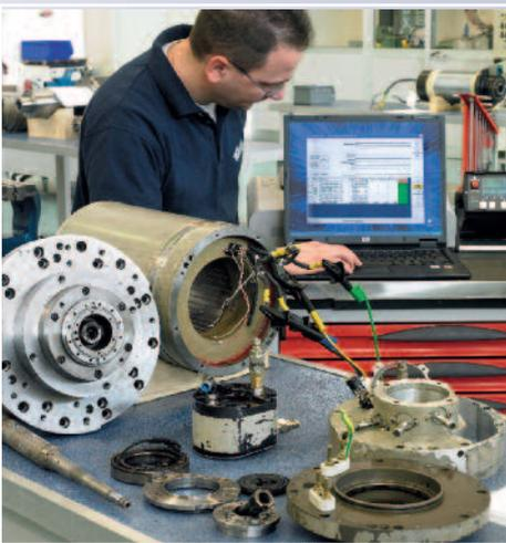
Check up of electric components, measurement of the parts, defect analysis and writing of the repair report.
