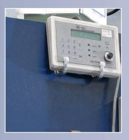
Fully automated test run with measurement and monitoring of temperature, greasing, drive and vibrations up to 180.000-1min using nominal current up to 250A for synchron- and asynchron motors.
