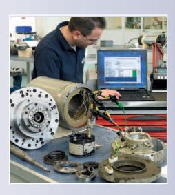
Check up of electric components, mesurement of the parts, defect analysis and writing of the repair report.
